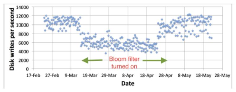
Figure: "Using a Bloom filter to prevent one-hit-wonders from being stored in a web cache decreased the rate of disk writes by nearly one half, reducing the load on the disks and potentially increasing disk performance."
